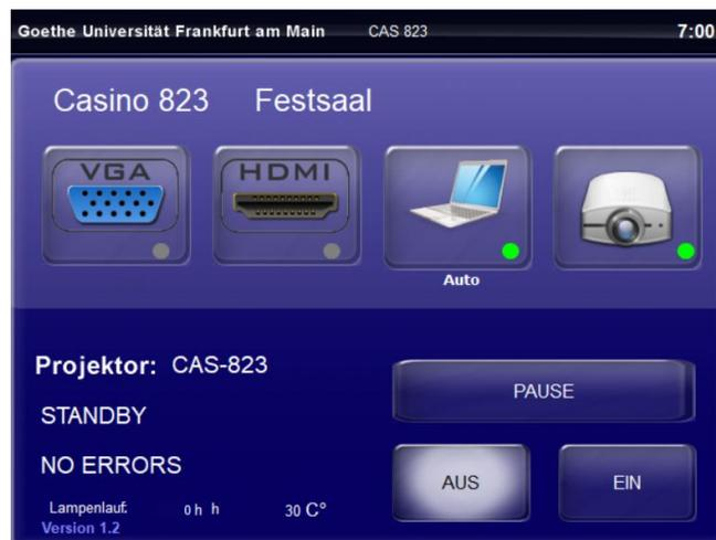
After establishing your Laptop connection you can determine which signal the projector receives and displays via the touch panel on the wall (shown above). Here you also have the option to 'pause' the projection or switch the projector off completely.
